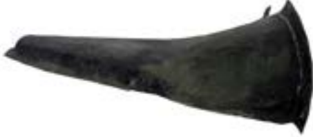
T-56 Transmission Tunnel 68-76
